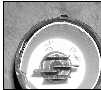
Figure 4: Flask assembly showing bead line up.
